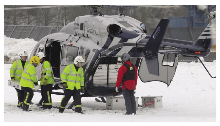
The ZARGES K470 universal case provides perfect protection, even under the most extreme conditions. The K470 is ATA 300 (Category 1) approved, UN Packaging Group 1 approved, lightweight, rugged, and dust and water resistant. Its durable construction provides optimal protection for any contents.
