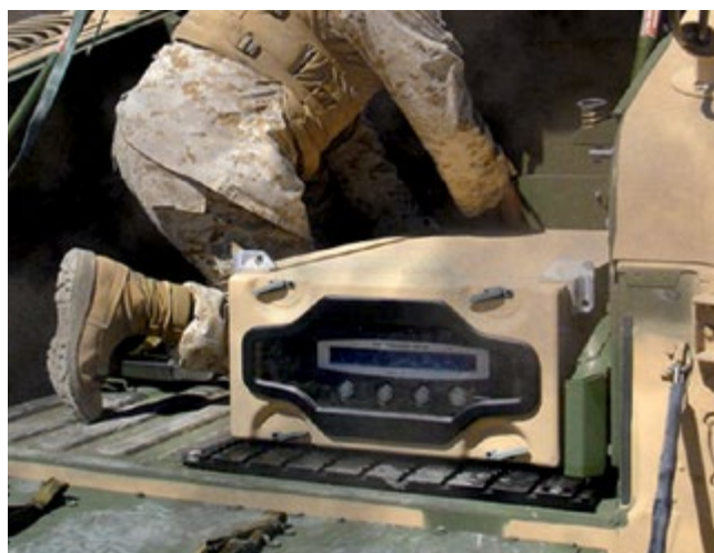
Anti-IED electronic system in Mitraset® Classic rackmount case with special reinforcement and custom cover, operated from a vehicle
