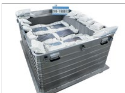
Inner packaging for lithium batteries with vermiculite pads and flame-retardant foam
