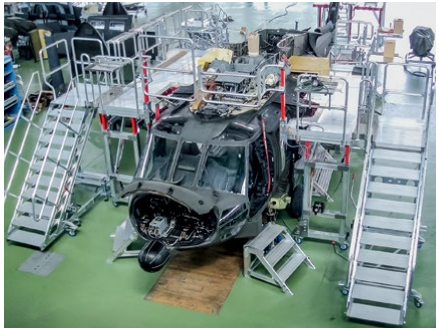
Height-adjustable work platforms that adapt to contours for optimal maintenance work
