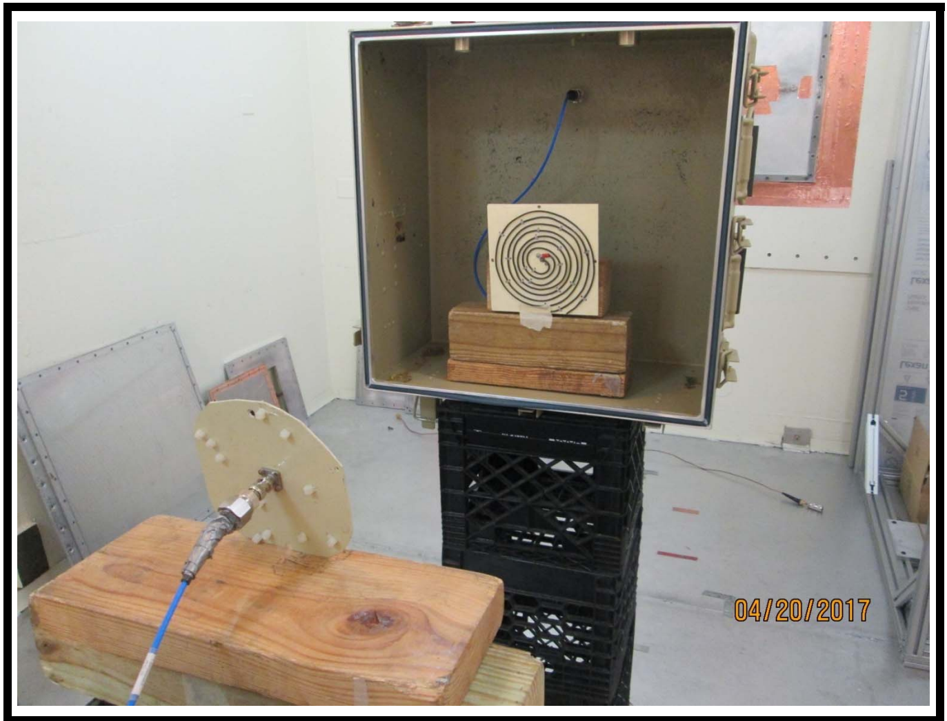
Photograph Description: Transmit Antenna Placement in Case (150kHz to 1GHz)
