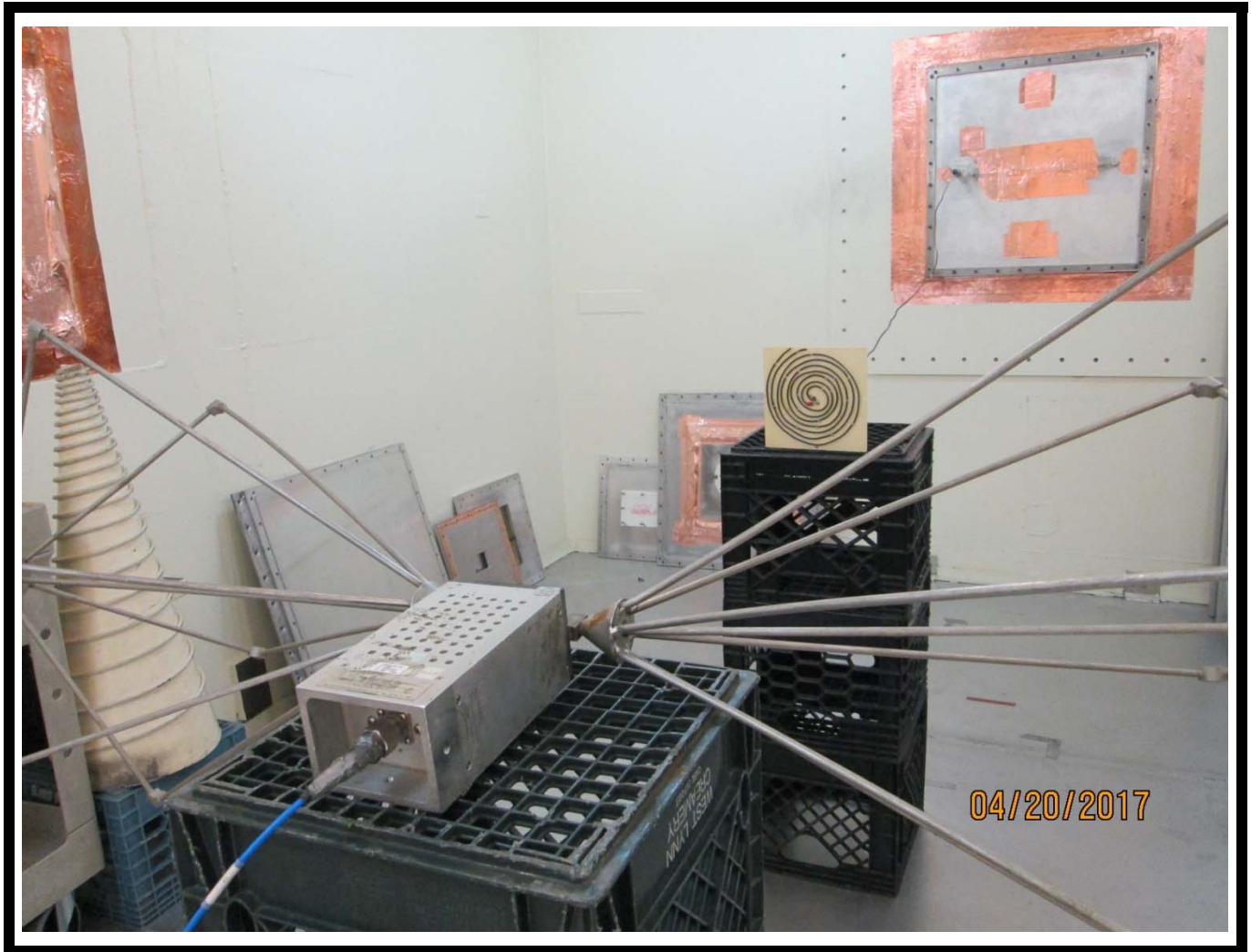
Photograph Description: General Open Reference Test Setup (Open Field)
