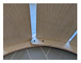
4. Next, use the Wooden and Metal Joint Locks to secure the two sides together. Push it in as far as you can and then screw it until it's tight. Avoid over tightening and stripping the screw.
