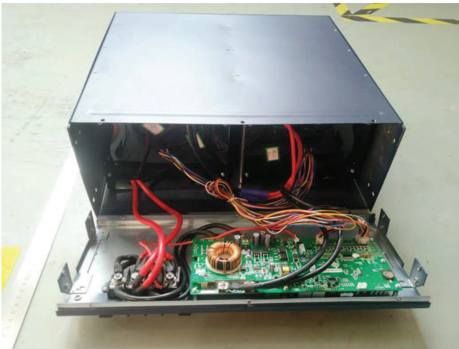
Pic.4 Internal View of Battery Module
