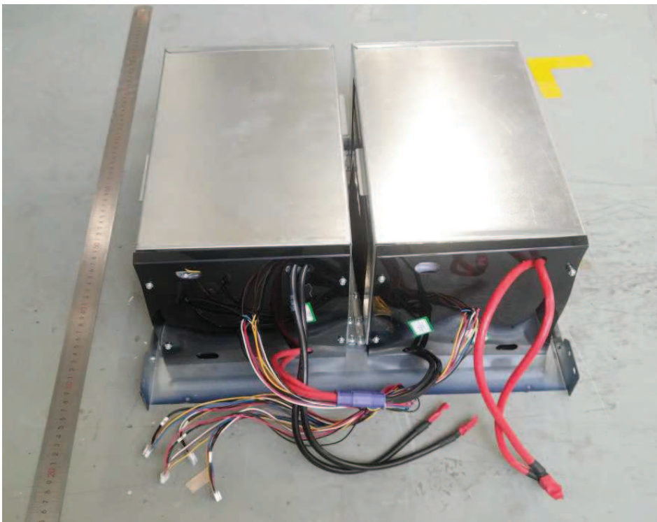
Pic.6 Internal View of Battery Module
