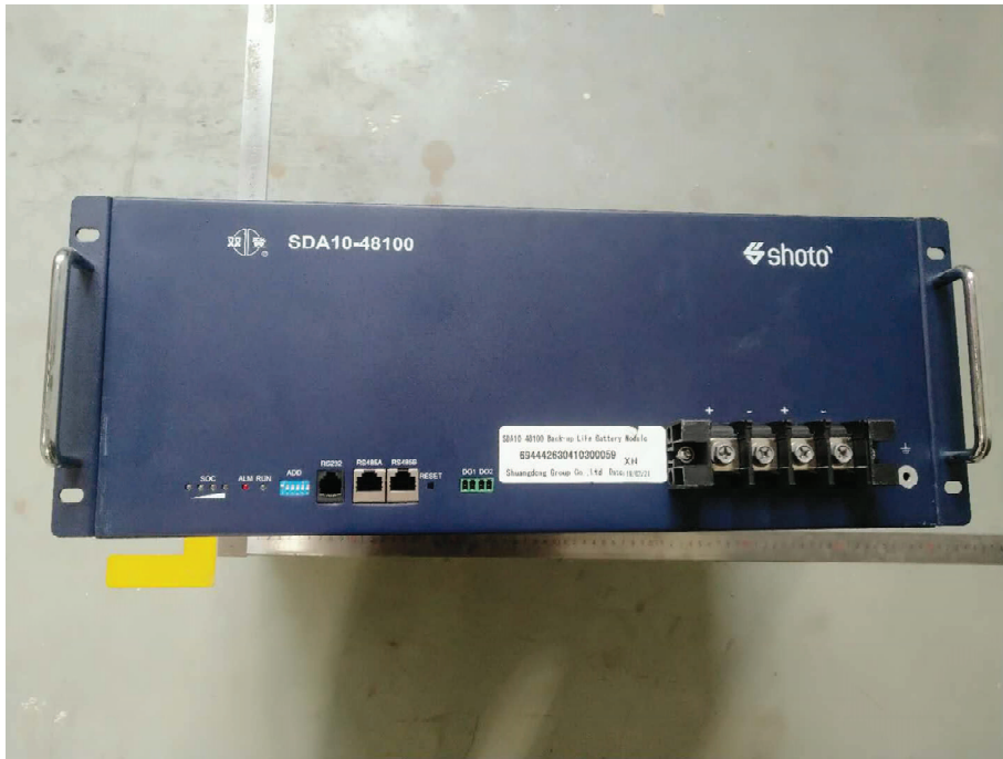
Pic.3 Front Terminal View of Battery Module
