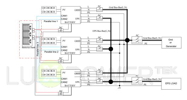
■ If you connect one battery bank shared by multiple inverters as the diagram above, please enable "Battery shared".
