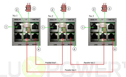
If there are more than three inverters parallel in this three-phase system, only two of the longest distance need to be dialed toward "on" position:  $1^{1}1^{1}$ , and others keep off:  $0^{1}0^{1}$
