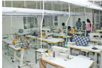
(https://1et31t3azwc3jxcfm1s69wb8-wpengine.netdna-ssl.com/wp-content/uploads/2015/03/Korra.jpg) The unit with 19 machines is run by 6 operators. At GCC, a denim jean has a throughput time of 4 hours
