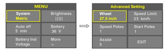
8.1 System : Press Up / Down button to switch between Metric / Imperial.
