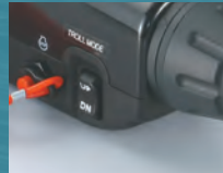
Troll mode switch activates SUZUKI Troll Mode System and controls RPM from idling engine speed up to 1200rpm at every 50rpm
