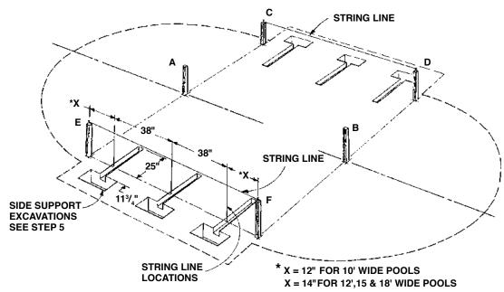
Locate Stakes C, D, E and F from your pool layout. Attach strings between C and D, then E and F. For 10' wide pools, the first side support excavation is positioned 12" ("X" dimension) from the center of either stake to the center of the excavation. For 12', 15' & 18' wide pools, the first side support excavation is positioned 14" ("X" dimension) from the center of either stake to the center of the excavation. All Pools: Other side support excavations are 38" center to center.
