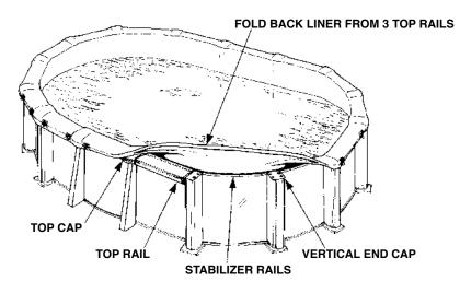
With the help of two or three people, raise and hold the liner up from any three top rail sections. Remove four top caps, three top rails, two vertical end caps and stabilizer rails. REMEMBER, NEVER ALLOW LINER TO FALL BACK INTO POOL.
