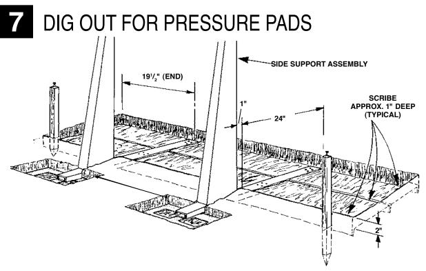
Dig out a trench to the dimensions shown above, grading to the ground support. Use a large screwdriver to scribe grooves (approximately 1" deeper) down each side and center of the trench to accomodate the pressure pads' flanges. Remove the excess dirt accumulated from scribing.
