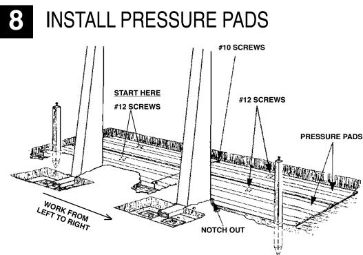
Keep the tops of the ground supports free of dirt. Working from left to right, assemble a set of pressure pads to each ground support using six (6) #12 x 3/4" screws as shown in Fig. A, (refer to your parts list as needed). Tighten screws firmly. Assemble each pressure pad set to its adjacent set using four (4) #10 x 1/2" screws. DO NOT OMIT ANY SCREWS.
