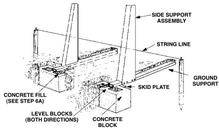
Remove string line. Place concrete blocks into the excavations as shown. **NOTE: The thicker wall side of the cement blocks must face up.** Level the blocks in both directions. Place the assembled side supports into each trench with skid plate resting firmly against the face of the concrete blocks. Check each ground support for level (refer to Step 6A).
