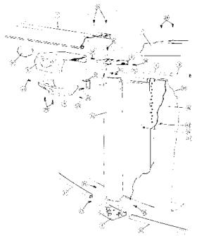
Attach brackets using all hardware shown. Refer to this illustration and your pool's parts list for parts identification.
