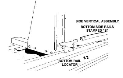
Loosely assemble bottom rails (stamped "S"), groove up, between verticals with bottom rail locators. Secure bottom rail locators to side verticals with screws. NOTE: Be sure to use the top set of holes in the side verticals when assembling the bottom rail locators.
