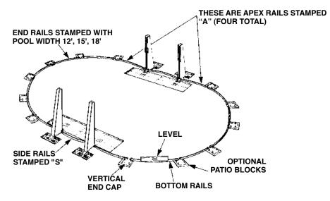
Begin ends of framework by installing the four rails to the outside of the end side verticals stamped "A". Complete ends by sliding bottom rails (groove up) into vertical end caps. Confirm levelness of installation by placing level on top of bottom rails. Check around the oval to be sure ground is flat and within 1 inch of level at opposite sides and ends of pool.
