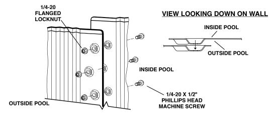
Bring the ends of the wall together and overlap them as shown. The raised feature on one wall end is received by the corresponding facing recess on the other wall end. **NOTE: If any adjustments are necessary to make the wall ends meet properly, make these adjustments equally at all bottom connectors.**
