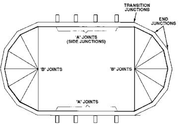
There are two top rails for each pool size. There are two different joints where the top rails meet as shown. Refer to Step 16 for attachment.
