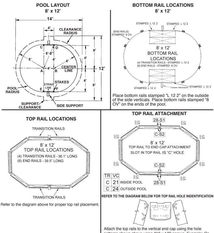
Attach the top rails to the vertical end cap using the hole patterns shown above using  $#10 \times 1/2$ " screws. Example: On the ends of the pool, attach top rail hole "C" to vertical cap hole "21" and top rail hole "C" to vertical cap hole "24".
