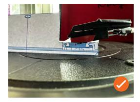
The side view paper model provides the understanding of the approximate placement of the stylus with the specific rubber support. It is compatible when the conditions mentioned above are met. If not, please try the other stylus support paper model.
