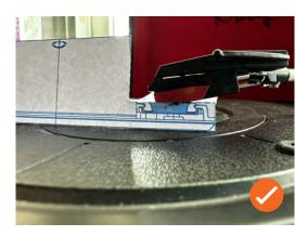
The side view paper model provides the understanding of the approximate placement of the stylus with the specific rubber support. It is compatible when the conditions mentioned above are met. If not, please try the other stylus support paper model.
