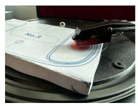
The top view paper model provides the understanding of the approximate size of the device, the diameter of the stylus supports and the height of the device.
