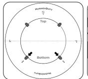
Insert the record into the gap of the **2 top** rubber stoppers.
