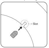
**4.** Push the **2 bottom** rubber **5.** stoppers toward the outer ring of the adapter.
