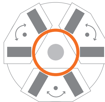
INOZet®での6点クランプ 6-point clamping with INOZet®
