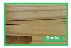
**Shake** appears like a series of splits. With a timber section of this size you will always encounter some degree of this (usually on one side). This does not affect the strength of the product and you will find the shake opens in continued warm weather and then closes up when the weather is wet and cooler or there is a lot of moisture in the air.
