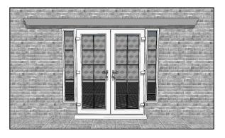
Work out where you wish to affix your wall plate, making sure that the area directly in front of it is flat, level and able to support the structure. Also check that the longer edge is at the top. Attach the wall plate using suitable fixings for the wall construction. Measure in 400mm from each end and use sufficient fixings so that the minimum distance between them is 500mm, distributed evenly and vertically centred across the wall. Ensure it is horizontal with a laser or spirit level.
