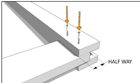
Take another post and slide it over the other (square) end of the runner so that it occupies half the width (around 47mm) of the slot in the post. Ensure it is square before securing in place with 2 of the 60mm screws
