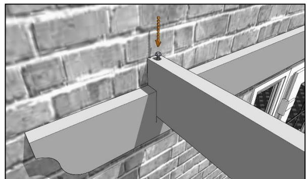
Make sure everything looks square and the rafter is aligned with the marks on the wall plate and fully slotted in place before securing into place with a 120mm coachscrew driven down through the rafter into the wall plate.
