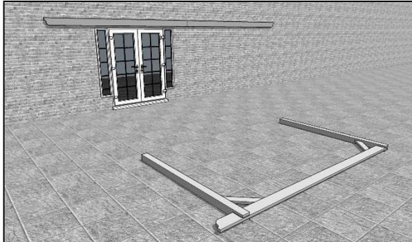
Get your assistants to manoeuvre the previously assembled "goalpost" assembly into place so that it is approximately in place, parallel to and about the length of a rafter away from the wall plate with the sculpted end outermost and opposite the sculpted end of the wall plate as shown...
