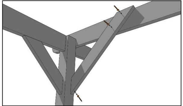
Now add the long braces, butting the angled face against the post and the bottom level with the short brace already installed. Fix the bottom end in place with a 70mm woodscrew and the top end in place with 2 of the 60mm woodscrews. Add the remaining 3 braces in the same manner.
