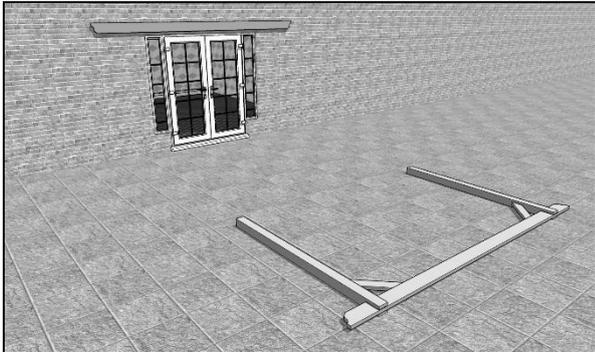
Get your assistants to manoeuvre the previously assembled "goalpost" assembly into place so that it is approximately in place, parallel to and about the length of a rafter away from the wall plate...
