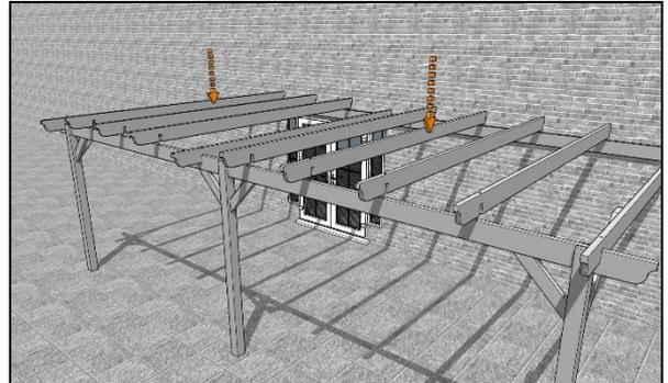
Finally, add the remaining rafters using the markings on the runners and wall plate as a guide, securing each one in place with a 120mm coachscrew down through each end, into the runner and wall plate.
