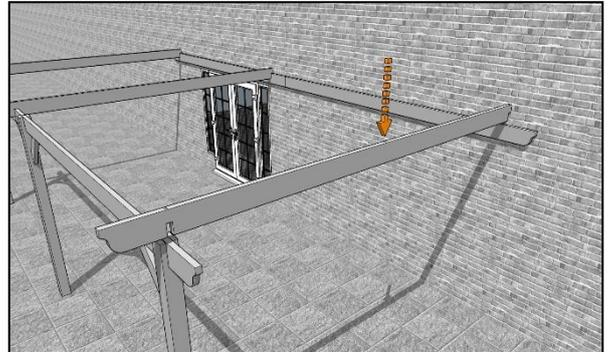
Now lower another rafter onto this end of the assembly, adjusting the post position if necessary, and once butted up to the outer face of the post and aligned on the wall plate marking, secure in place with a 120mm coachscrew at each end in the same way as you did for Steps 22 & 23.
