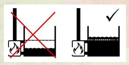
Figure 5: Necessary water level
