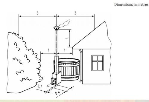
Figure 4: Minimum distances for firewood heated hot tub
