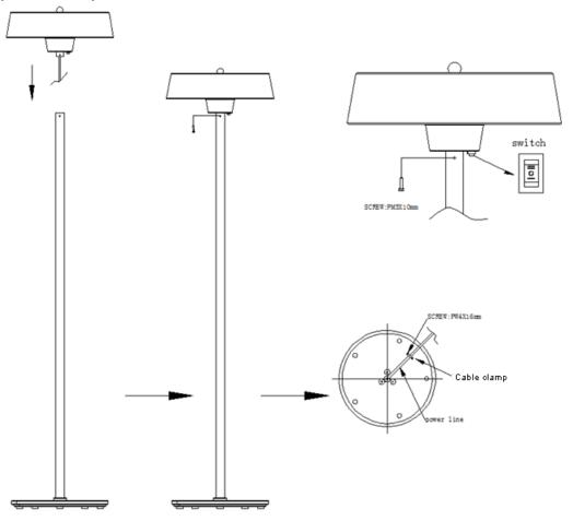
Step 3. Connect the plugged mains lead to the heater cable using the connector supplied
