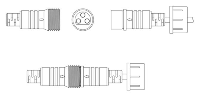
Attach the mains cable using the supplied connector and cable clamp. The connector is specially shaped so it only fits correctly one way. Screw both halves of the connector firmly together.
