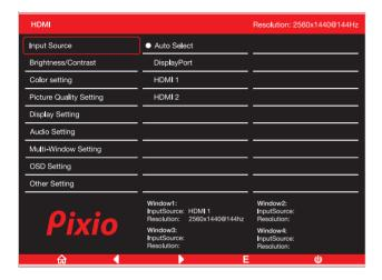
Switch the signal input to DisplayPort, HDMI 1, HDMI 2, or have the monitor Auto Select the source.
