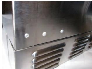
3. Loosen but do not remove the outer top and bottom screws on the right-side hinge.
