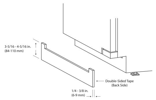
NOTE: When finishing the grill/plinth, be sure to stain the front, back and all edges to prevent warping.
