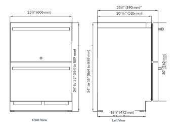
\*Dimensions are the same for Panel Ready unit when ¾" panel applied
