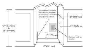
NOTE: For Gravity drain models, the drain hole cannot exceed 7 inches above the floor. For Pump models, the drain hole should be no lower than 7 inches and no higher than 4 feet above the floor.
