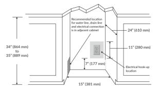
NOTE: For Gravity drain models, the drain hole cannot exceed 7 inches above the floor. For Pump models, the drain hole should be no lower than 7 inches and no higher than 4 feet above the floor.
