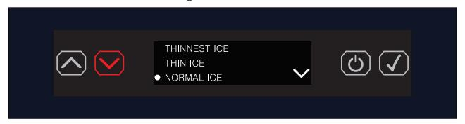
6. Press the DOWN ARROW button ( ) to scroll to the desired setting.
