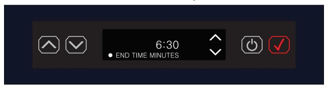
24. Using the UP / DOWN arrow button select END TIME AM or PM and the AM / PM will flash until the user makes a selection.
