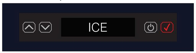
2. Scroll down to TURN ON QUIET 4 HOURS setting and press the ENTER button ( ).
