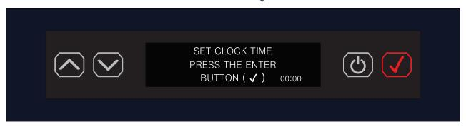
5. The display will show the clock at 00:00 and prompt the user to set the hour with the hour position flashing the 00.
