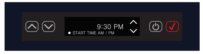
19. Once the START TIME is properly set, the display prompts the user to set the END TIME HOUR for the SCHEDULE QUIET MODE pressing the UP or DOWN arrow and the display will show the hours section flashing 00.
