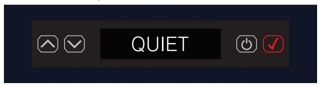
2. Scroll down to TURN OFF QUIET 4 HOURS setting and press the ENTER button ( ).
