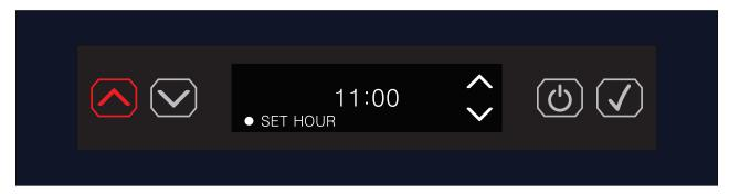
7. Once the HOUR is set, press the ENTER button ( ) and the display will show the minutes position blashing the 00.
