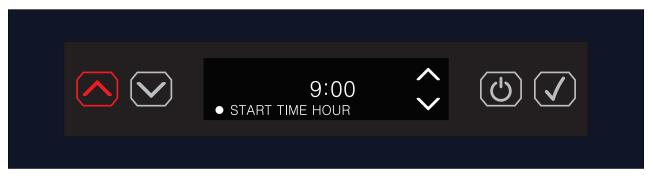
14. Once the HOUR is set, press the ENTER button ( ✓ ) and the display will show the minutes section flashing 00.
