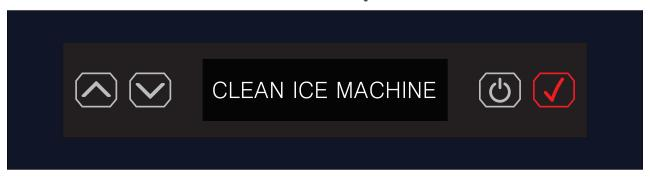
2. To CONFIRM the CLEANING function, press the ENTER button ( ✓ ) again.
