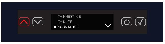
Press the ENTER button ( ✓ ) to scroll to desired setting.
