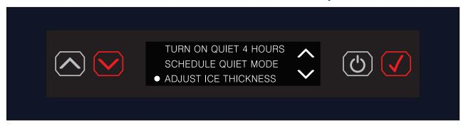
3. Press the UP or DOWN ARROW button ( ) to scroll to desired setting.
