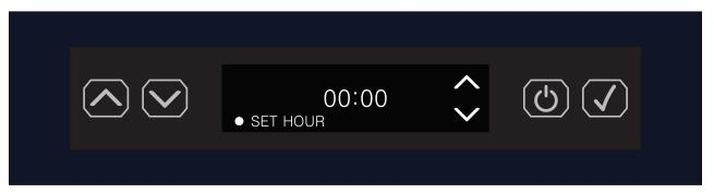
6. Using the UP / DOWN arrow button set the HOUR.
