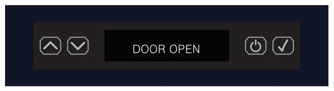
NOTE: The audible alert is 3 beeps that occur every 30 seconds after the door has remained open for more than 2 minutes and automatically clears when the door is properly closed. This methodology applies to any error or alert that requires an audible alert.
