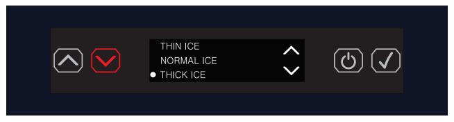
7. Press the DOWN ARROW button ( ) to scroll to the desired setting.
