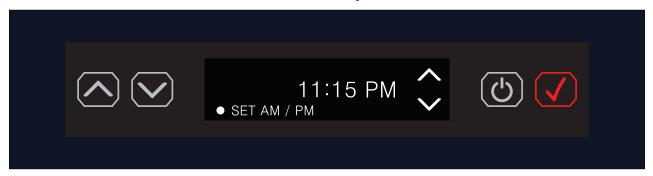
12. Once the time is properly set, the display prompts the user to set the START TIME HOUR for the SCHEDULE QUIET MODE pressing the UP or DOWN arrow and the display will show the hour section flashing 00.
