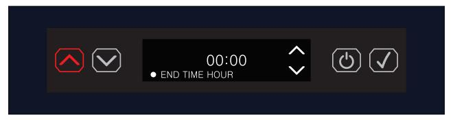
20. Using the UP / DOWN arrow button select the END TIME HOUR.
