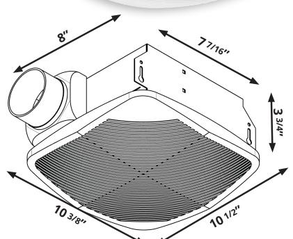
UL Listed for use over bathtubs and showers when connected to a GFCI protected branch circuit (ceiling mount only).
