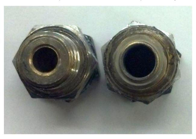
The ID on the LEFT fitting is approximately 5mm. It is for the OLD Style Stainless Steel sphere, which was eventually replaced by the Teflon mushroom.
