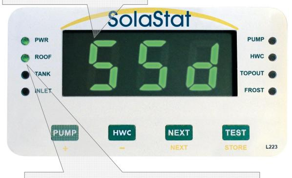
When **SSd** is displayed, the **ROOF**, or **TANK** light will be on or flashing to indicate which sensor is faulty. In this case, a faulty **ROOF** sensor has been detected.
