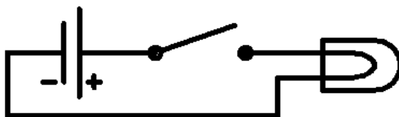
Figure 5-3: Schematic Drawing of Flashlight
