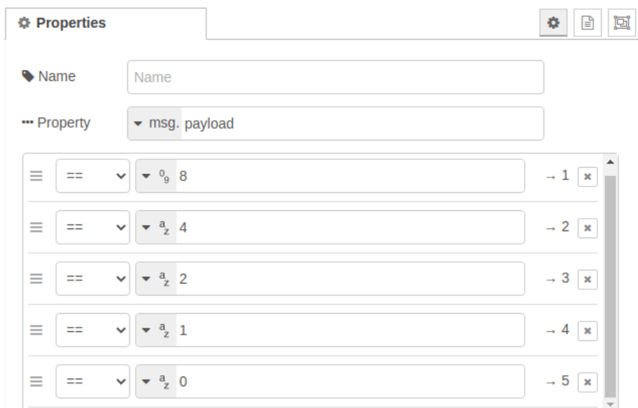
Figure 4-68: Shifting Lights Flow Switch Node Edit
