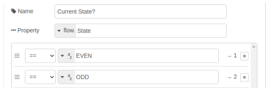
Figure 6-31: Finite State Machine - Current State Evaluation
