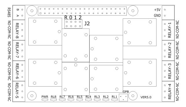
Your 8-RELAYS card comes with appropriate mounting hardware. Up to eight 8-RELAYS cards can be stacked on top of one Raspberry Pi. Eight LEDs indicate the status of their respective relay. An LED is lit when the corresponding relay is energized. The General Purpose Pushbutton GPB is connected to pin 37 of the Raspberry Pi GPIO connector (GPIO26). In order to use the pushbutton you need to write a shell script to accomplish the desired function.
