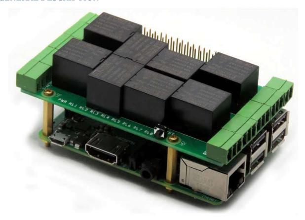
The 8-RELAYS card is a stackable expansion card for Raspberry Pi. The card is compatible with all Raspberry Pi versions from Zero to 4. It offers a compact and inexpensive solution for adding up to 64 relays to your Raspberry Pi project.
