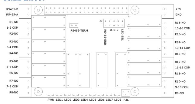
Your 16-RELAYS card comes with appropriate mounting hardware. Up to eight 16-RELAYS cards can be stacked on top of one Raspberry Pi. Eight LEDs indicate the status of their respective relay. An LED is lit when the corresponding relay is energized. The General Purpose Pushbutton GPB is connected to pin 37 of the Raspberry Pi GPIO connector (GPIO26). In order to use the pushbutton you need to write a shell script to accomplish the desired function.
