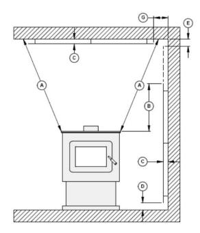
Figure 13: Heat shield clearances
