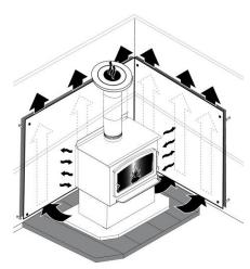
It is often desired to use as little space as possible when installing a wood stove. To do this, it is possible to reduce the clearances safely and install the stove closer to the walls by permanently installing a heat shield between the stove and the flammable material.
