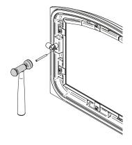
Figure 15: Installing the split pin
