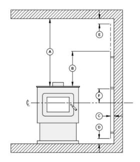
Figure 12: Heat shield clearances
