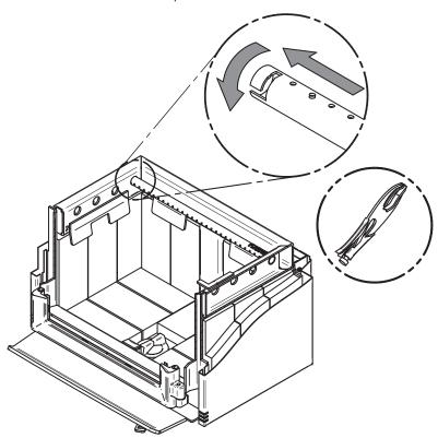
Note that secondary air tubes **(B)** can be replaced without removing the baffle board **(A)** and that all tubes are identical.
