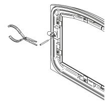
Figure 14: Removing the split pin
