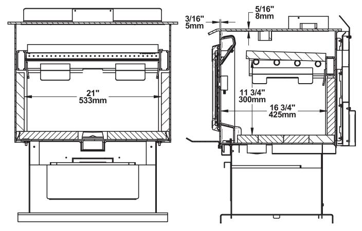
Figure 5: Front View - Combustion Chamber
