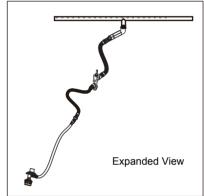
Orifice is located in this connection
