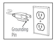
A 15 Amp, 120 Volt circuit is required. A dedicated circuit is preferred, but not essential in all cases. A dedicated circuit will be required if, after installation, the circuit breaker trips or the fuse blows on a regular basis when the heater is operating. Additional appliances on the same circuit may exceed the current rating of the circuit breaker.
