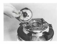
2. Place a few drops of Filter Queen Oil of Pine or Oil of Eucalyptus on grey felt Air-Scent Pad. CAUTION: Do not saturate or use perfume or other liquid not sold by HMI Industries, Inc.! Use of other liquids could cause damage to your motor and void your warranty. (To replace felt Air Scent Pad, twist clamp to the left and lift off; insert new Pad. Replace clamp, lock in position.)
