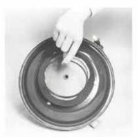
2. After removing the Cone Guard, the Secondary Filter is fully exposed. To remove it, pull back the plastic Retainer Ring with your finger and lift out. The Filter can now be removed.
