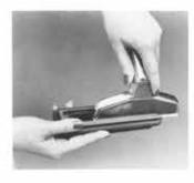
Assemble Filter Queen for cleaning and other Attachments. Cleaning overstuffed furniture, mattresses, fabrics: To remove deeply imbedded dirt in heavy fabrics, use the Six-Inch Nozzle without Brush. Use the Brush when fabric is covered with threads, lint, etc. When cleaning mattresses, upholstered furniture, clothing and other off-the-floor objects, attach Nozzle directly to the Hose.
