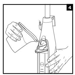
4 Use the filling flask to pour distilled water into the tank. Make sure to not exceed the Max Fill line on the flask. When finished, close the tank lid firmly.
