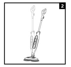
2 To start cleaning, step on the nozzle and pull the handle towards you. This will engage the power pads.
