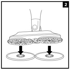
2 To attach the Dirt Grip™ or Dusting pads, place **BOTH** pads flat on the floor with the plastic rings facing up. Align the indentation on the rotating discs on the bottom of the nozzle with the plastic rings on the pads, then gently lower the nozzle onto the pads, pressing until the pads are secured.
