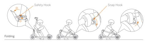
Turn off your KickScooter. Turn the safety hook counterclockwise and open the guick release lever.
