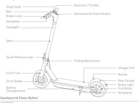
Speedometer: Display the current speed of the KickScooter, as well as to display error codes.
