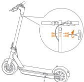
Firmly connect the wires inside the handle and the stem. Slide the handle onto the stem. Be aware of the correct orientation.
