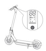
Power on the KickScooter and check the power level indicator. Charge the KickScooter if the battery level is low.
