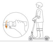
3. Put your other foot on the footrest to keep both feet stable. Press the throttle on the right hand to speed up when you are balanced.
