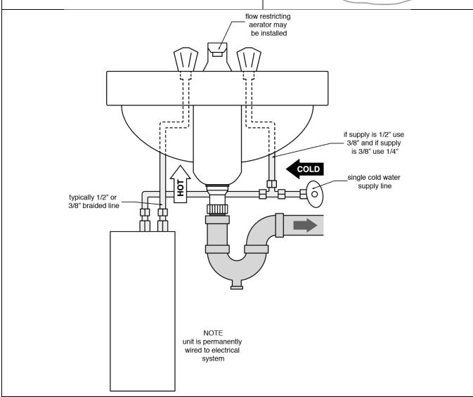
**4.** Open the hot water faucet and run water for minimum 60 seconds and until the flow is continuous and free of air pockets. Close the faucet and install the aerator (if supplied).
