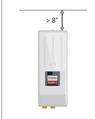
**3.** Remove the cover and fasten to the wall using the four mounting holes at each corner of the back plate. Replace the cover.
