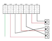
IF YOU MEASURE VOLTAGE ACROSS ONE OF THE LEGS IN A SET AND VOLTAGE IN ANOTHER LEG OF ANOTHER SET, THEN YOUR WIRES AT THE BREAKERS ARE CROSSED AND MUST BE CORRECTED. EXAMPLE-L1-L1 READS NO VOLTAGE, BUT L1-L2 GIVES YOU VOLTAGE READING, THEN YOUR WIRES AT THE BREAKERS ARE CROSSED AND MUST BE FIXED.
