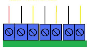
CHECK THE FUSE USING YOUR VOLT METER. PLACE ONE PROBE ON THE FARTHEST LEFT TERMINAL BLOCK THAT HAS THE **RED** FUSE WIRE CONNECTION AND THE OTHER PROBE TO GROUND. YOU SHOULD GET A VOLTAGE READING OF 110-120V, IF THERE IS NO READING THE FUSE MUST BE REPLACED.
