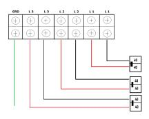
DISCONNECT ALL BREAKERS AT THE SERVICE PANEL. ONCE ALL BREAKERS HAVE BEEN DISCONNECTED MEASURE THE VOLTAGE GOING TO EACH ONE OF THE SETS (L1 L1) (L2 L2) (L3 L3 ) ALL SHOULD READ 0 VOLTAGE.
