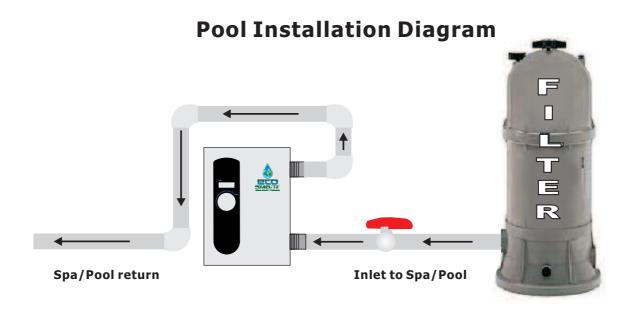
SHUT OFF VALVE MUST BE INSTALLED AT INLET OF UNIT. ELECTRICAL AND PLUMBING CONNECTIONS MUST BE FOLLOWED TO MEET ALL LOCAL CODES AND REQUIREMENTS.
