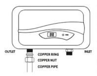
This water heater is supplied with 1/2" compression fittings, Do not weld or use Teflon or paste.
