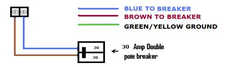
IF POWER GOING TO THE UNIT IS NOT CORRECT, THE UNIT WILL NOT OPERATE CORRECTLY, SO IT IS IMPORTANT TO PERFORM THIS TEST FIRST, BEFORE PROCEEDING .
