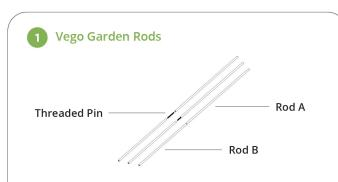
Vego Garden bracing rods are used to reinforce the strength of oversized raised beds. For 2ft wide raised bed: use Rod A only; For 3.5ft wide raised bed: use the threaded pin to assemble Rod A & Rod B.
