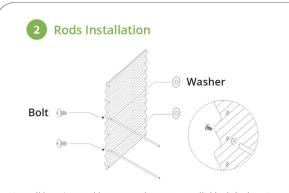
Install bracing rod between the two parallel bolt holes. Attach bolt, panel, washer & rod loosely, making sure that the rods are connected to the **third** and **fifth** bolt holes from the top. Then tighten them up by screwdriver for reinforcement of raised bed.
