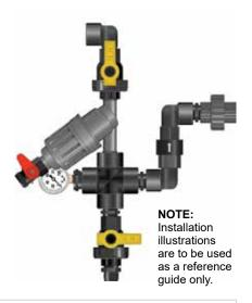
HYKSTART-DAB Kit is to be used with any Booster Pump that regulates the pressure (not to exceed 85 psi). If the pump being installed does not regulate the pressure to the system specifications, a regulator is necesary.
