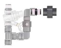
Attach the last **Elbow** to the top of the **Check Valve**.
