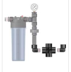
7 To the bottom of the Cross, attach a Close Nipple, the Banjo<sup>®</sup> Ball Valve, and the Hose Adapter.
