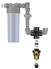
To the Elbow on the right, attach a Reducer Nipple, the 1" Tee, and the other Reducer Nipple, in that particular order.
