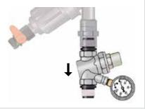
7 Connect the Tee to the other end of the Pressure Regulator assembly.
