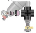
To the right of the Cross install the four pieces that form the Check Valve Assy (4" Nipple, Check Valve, Close Nipple, and Union).
