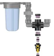
To the **Elbow** on the right, attach a **1 1/2" Close Nipple**, the **Tee**, and the last **Elbow**.
