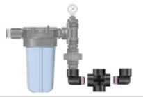
In the top opening of the Cross, insert a 1 1/2" to 3/4" Reducer Bushing.
