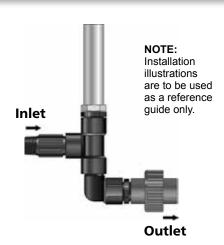
Wrap 5 to 6 turns of **Teflon<sup>®</sup> tape** on all threads. Make sure to wrap tape clockwise to prevent from unravelling.
