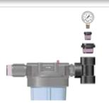
To the bottom opening of the Tee, attach a 1 1/2" Close Nipple, a Union, another 1 1/2" Close Nipple, and an Elbow (with the threads facing to the right), in that particular order.
