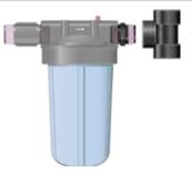
Attach a 1 1/2" to 3/4" Reducer Bushing, a 3/4" to 1/4" Reducer Bushing, and the Pressure Gauge, to the top opening of the Tee.
