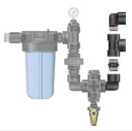
Insert the 1 1/2" to 1" Reducer Bushing in the middle opening of the Tee.
