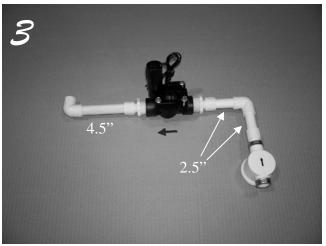
Using PVC glue assemble the pieces as shown above. System is designed for filter to overhang the bench edge.
