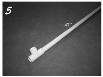
Continue installing the 48" pieces and the T fittings. The middle leg on all T fittings must face up.
