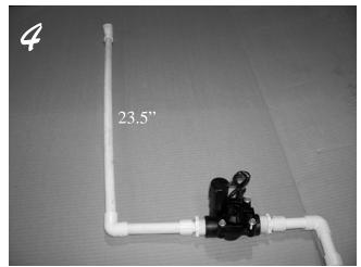
Connect the first piece of tubing to the elbow and install the T fitting with the middle leg pointing straight up.
