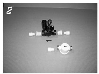
Thread fittings & adapters into both sides of the solenoid (watch for flow arrows) and the outlet side of the filter. Use Teflon tape on these fittings. Tighten securely to prevent leaks. *Great care must be taken to keep the glue out of the solenoid valve.*
