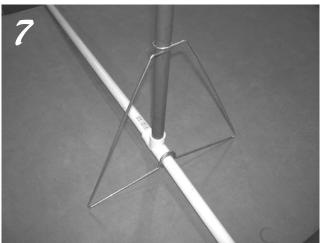
Install the gray risers by gluing them into the T fitting. The Irrigation stands are used 1 at each end and 1 (or more) spaced down length. Every upright does not receive a stand.
