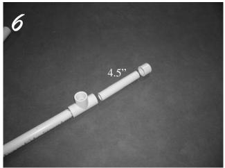
After all of the T fittings and 48" pieces are assembled the end can be capped. Glue the tail extension in place and cap. The extension is used to allow for further expansion by cutting the cap off and using a coupler to attach additional length.
