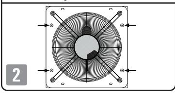
Using appropriate hardware (not provided) for your structure and the weight of your exhaust fan, secure the fan to your structure using the (8) pre-drilled holes on the flange. Exhaust fan must be mounted with the motor inside of structure, protected from the weather, and with capacitor on top as shown.
