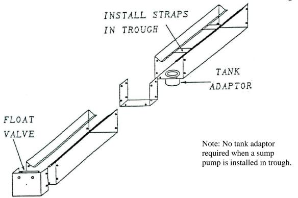
Place the mastic strips inside of the u connector and bolt together with the trough.
