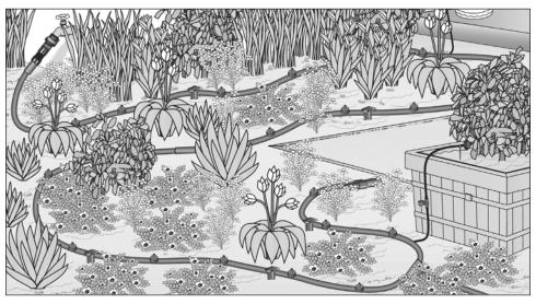
This kit can be connected into a 3/4" faucet/spigot or at the end of a garden hose. If a faucet is not adjacent to the garden or to the location of the installation, you may extend from the faucet using a garden hose or an additional length of 1/2" drip tubing (model B35 for 50' or B36 for 100').
